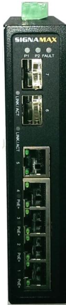
Figure 2.2: The Front Panel of 065-7407GPOEP
