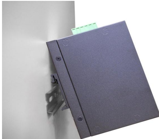
Figure 3.2: Insert the Switch on the DIN-Rail
