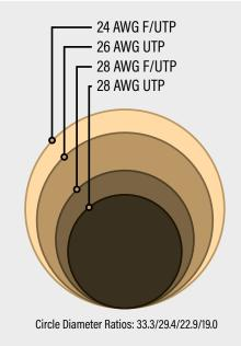
Unscreened 28-AWG cords provide certain advantage in cable size (therefore, flexibility and weight) compared to 26-AWG counterparts at expense of significant reduction in length; screened 28-AWG cords due to additional thickness of screening elements are not found that attractive. Overall, cost reduction looks like the biggest gain in switching to 28-AWG cords due to the copper content being 40% lower compared to the 26-AWG cords.
