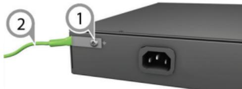
1. Ensure the rack is properly grounded and in compliance with ETSI ETS 300 253. Verify that there is a good electrical connection to the grounding point on the rack (no paint or isolating surface treatment).
