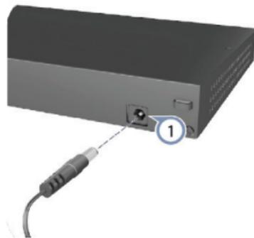
**Note:** The switches includes an AC/DC power adapter. Connect the AC/DC power adapter to the switch and to an AC power source.
