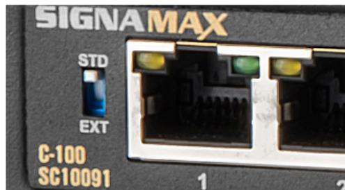
1. Extend mode provides PoE and 10Mb Ethernet to standard clients up to 250m (820ft) without any additional hardware. Downlink ports are isolated to only allow communication with uplink ports.
