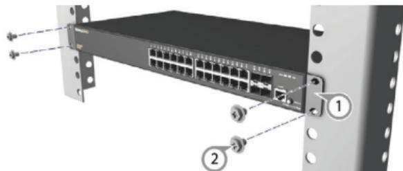
1. Attach the brackets to the switch.
