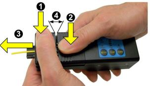
This operation may require some training in order to determine force that should be applied to heater's cover. Excessive force may break fiber, weak grip may result in poor stripping.
