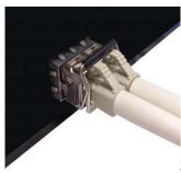
2. Connect the optical fiber (1/2 core) to the LC connector(s) of the SFP.
